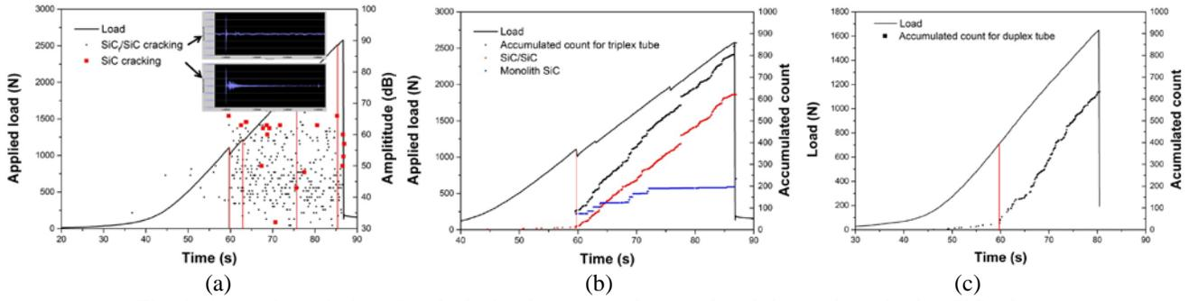
Fig. 1. Acoustic emission signals during hoop tests for (a), (b) triplex and (c) duplex SiC tubes.
