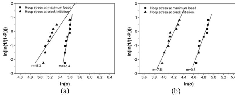
Fig. 2. Weibull distribution of the multi-layered SiC composite tubes: (a) triplex and (b) duplex SiC tubes.
