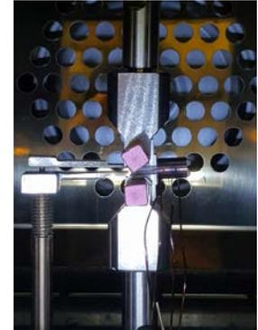
Fig. 5. Pictures of DHC crack and test set-up.
