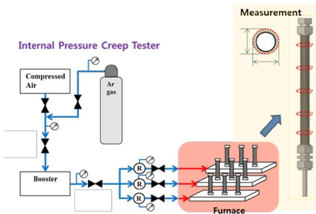
Fig. 2. Creep tester and test methods.
