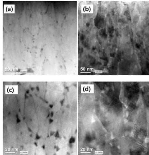
Fig. 2 (a) (c) Dark field STEM image of an area in the outer part of oxide showing the interlinked porosity. (b) (d) is Bright field STEM image of (a) (c).
