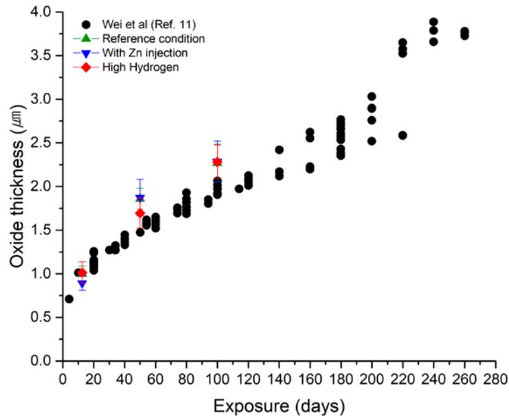
Fig. 1. Comparison of the average oxide thickness under each condition and with another study (Ref. 11). The values of the oxide thickness of 100 days corroded- samples were measured by SEM, and the 300 hours and 50 days corroded sample's oxide thickness were measured by STEM image.
