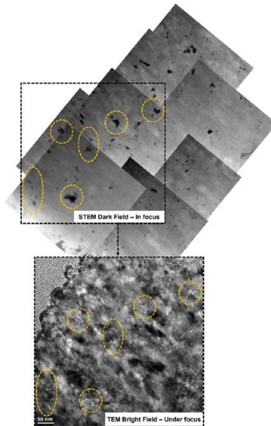
Fig. 3 Comparison of the STEM image (Dark field) and the TEM under-focusing image (Bright field) at the same locations for the 100 days corroded- sample in Zn injection condition (Orange circles indicate the same location).
