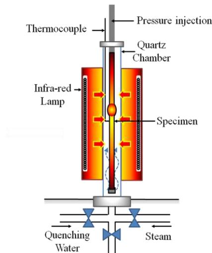
Fig. 1. Schematic illustration for the integral LOCA apparatus.
