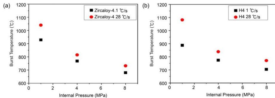
Fig. 3. Burst temperature as a function of internal pressure for (a) Zircaloy-4 and (b) H4 cladding specimens.
