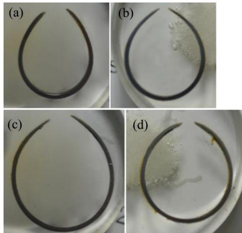
Fig. 4. Cross-sectional optical micrographic images at burst midplane for (a) as-received H4 cladding with heating rate of 28 °C/s, (b) prehydrided (300 wppm) H4 cladding with heating rate of 28 °C/s, (c) as-received H4 cladding with heating rate of 1 °C/s, and (d) prehydrided (300 wppm) H4 cladding with heating rate of 1 °C/s.
