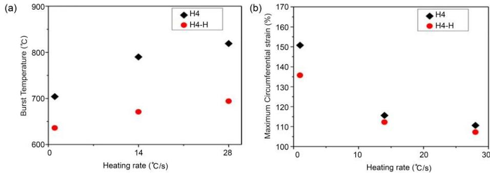
Fig. 5. (a) Burst temperature and (b) maximum circumferential strain as a function of heating rate for H4 and H4 cladding specimens.
