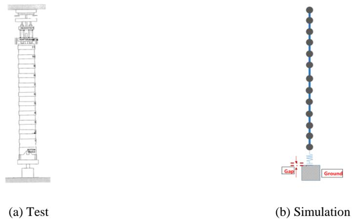
Fig. 6 Axial drop test setup and simulation model constitution
