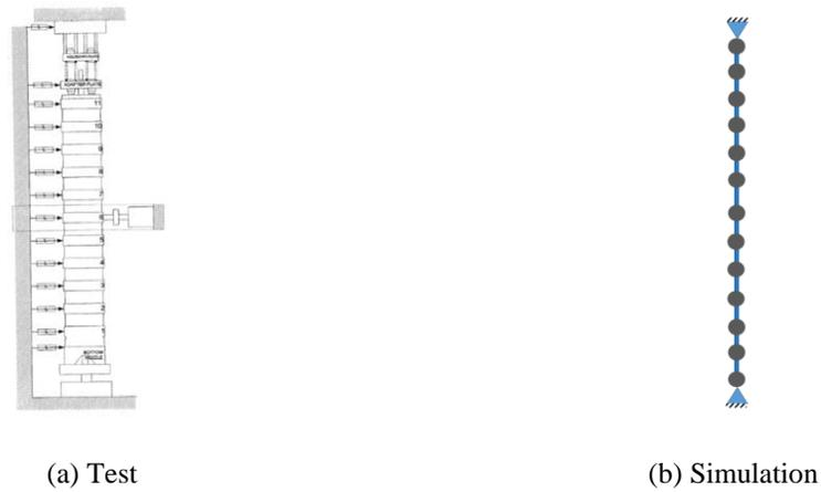
Fig. 4 Lateral vibration test setup and simulation model constitution
