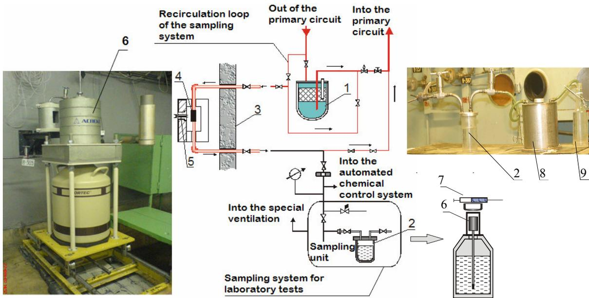
Fig. 1. Outfitting scheme of the PV-1 loop facility primary circuit at the MIR reactor and its completion with measuring equipment: 1 – ion-exchange filter; 2 – displaceable sampling tank; 3 – wall of the PV-1 loop facility shielded chamber; 4 – measuring tank; 5 – collimator; 6 – detector; 7 – syringe with a sample; 8 – gas delay tank; 9 – water tank.
