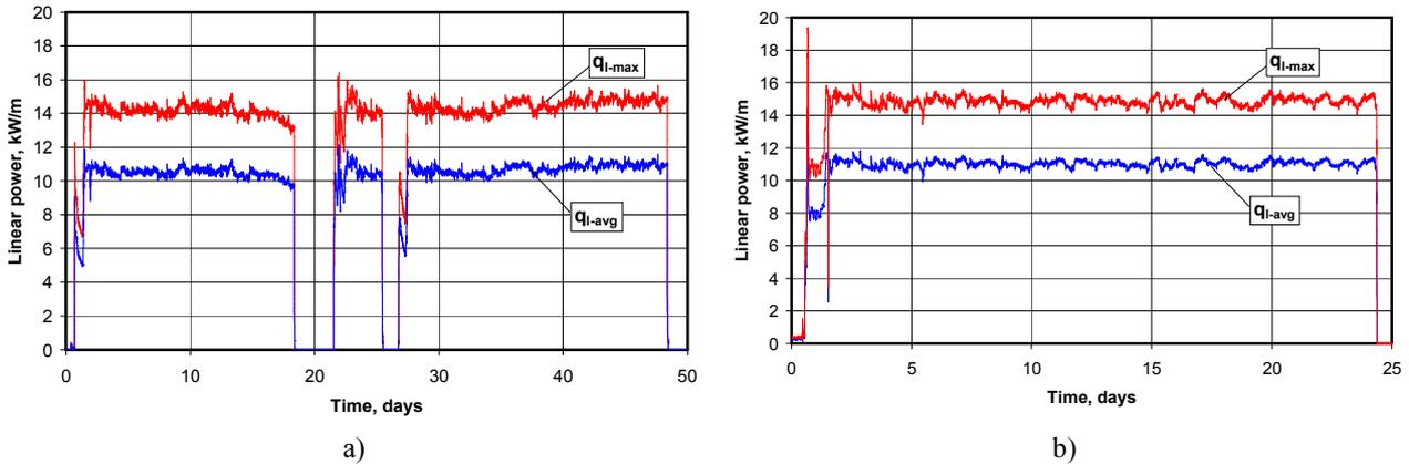
Fig. 3. Peak and average linear power of fuel rod with artificially applied defect during irradiation test # 1 (a) and # 2 (b).
