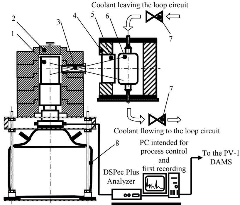
Fig. 2. Layout of the PV-1 loop facility coolant gamma spectra measurement area at the MIR reactor:
