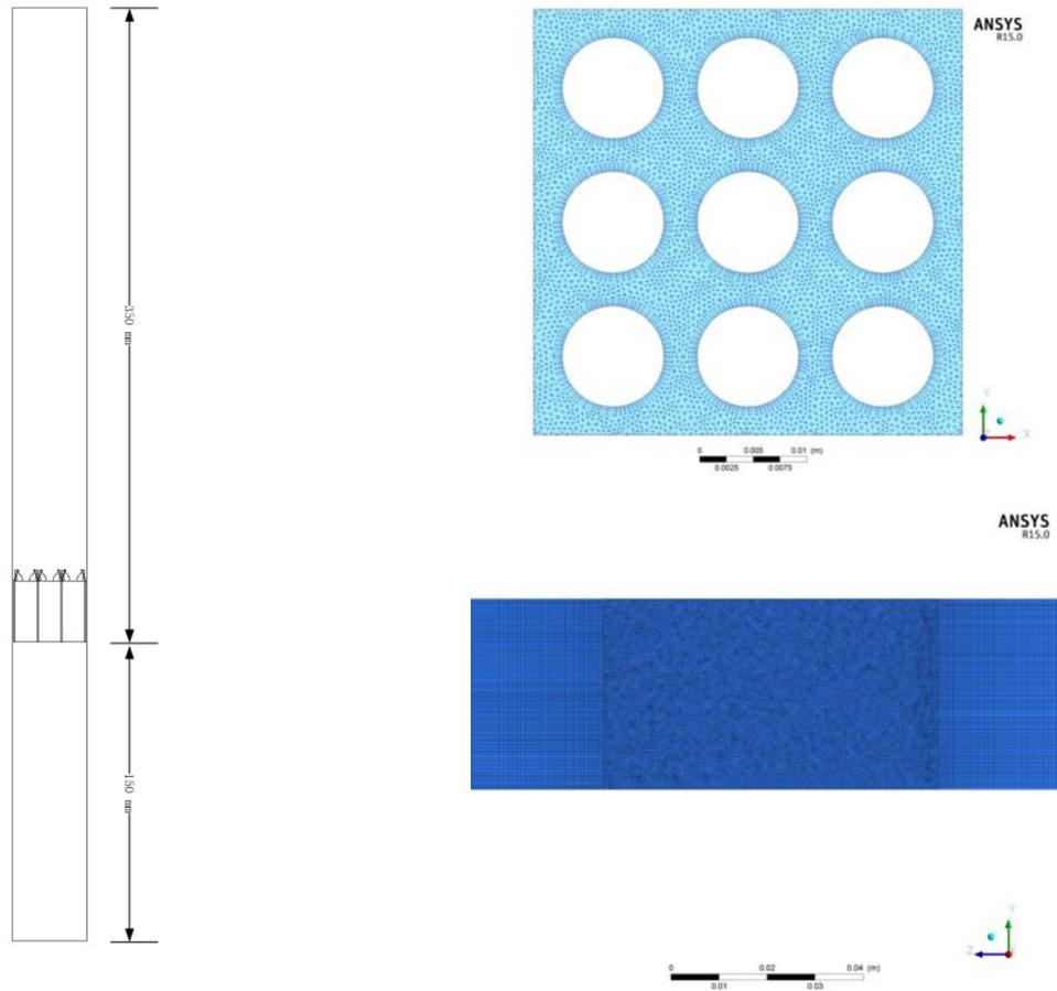
Figure 1. The calculation region and mesh
