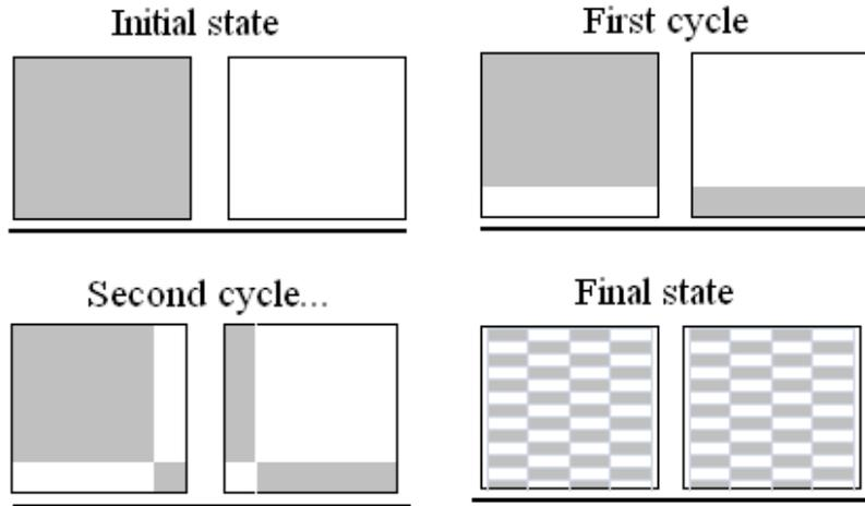
Fig. 5. Transition of phase volumes from an initial state with completely divided phases to final with uniform and identical distribution of phases in both volumes.
