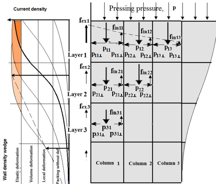
Fig. 9. Splitting a pellet into final elements, action of pressing forces in them, distribution of density
