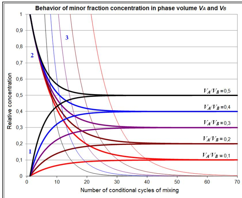
Fig. 6. Behavior of concentration of one fraction (minimal) depending on part of mixing  $k$ , and fraction volume relation of  $V_a/V_b$ . Three families of curves are given in drawing: 1 and 2 - concentration of a minimal phase in one and other phase volume; 3 - a difference of concentration of phases in different phase volumes.
