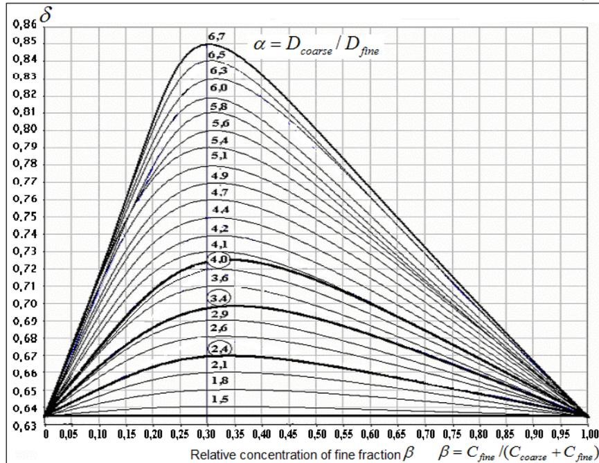
Fig. 4. Chart of packing of two any mono-fractions
