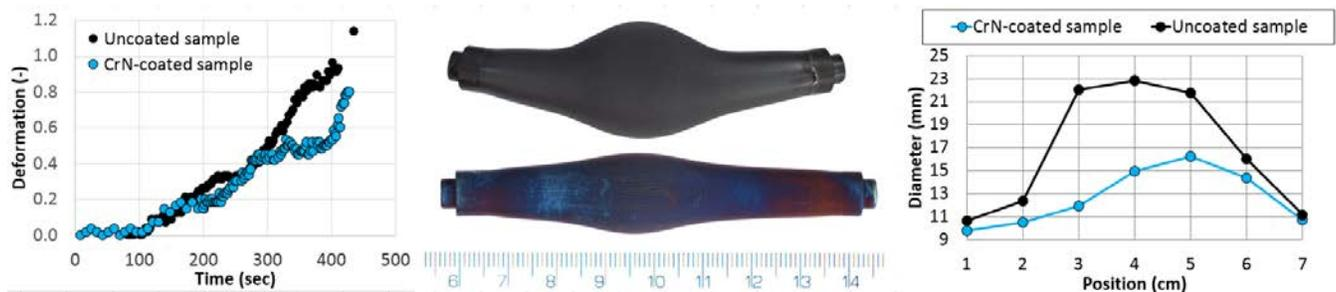
Figure 3: Left: development of deformation during burst test; Center: image of CrN-coated (down) and uncoated sample (up); Right: diameter of CrN-coated and uncoated sample after burst test in several positions.
