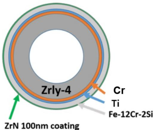
Fig 2. Schematic of the proposed MMLC
