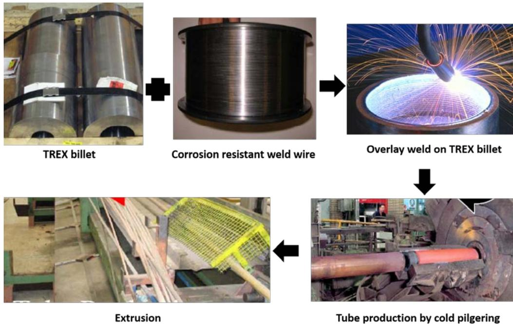
Fig 3. Example of MMLC cladding production process fabricated from welding and pilgering
