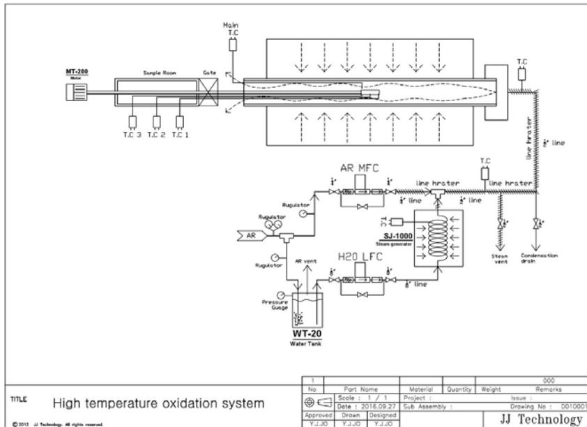
Fig 4. Schematic of high temperature oxidation steam furnace
