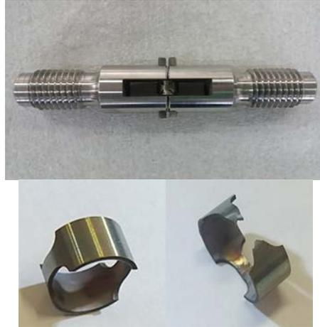
Fig 6. Ring tensile test sample holder(top) and samples before and after tensile test(bottom)
