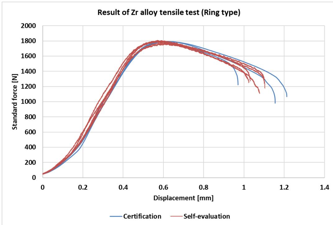
Fig 7. Result of ring tensile test of ref. zirconium alloy (at room temperature)
