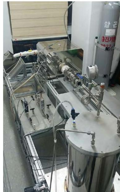
Fig 5. High temperature oxidation steam furnace schematic(left) and reality (right)
