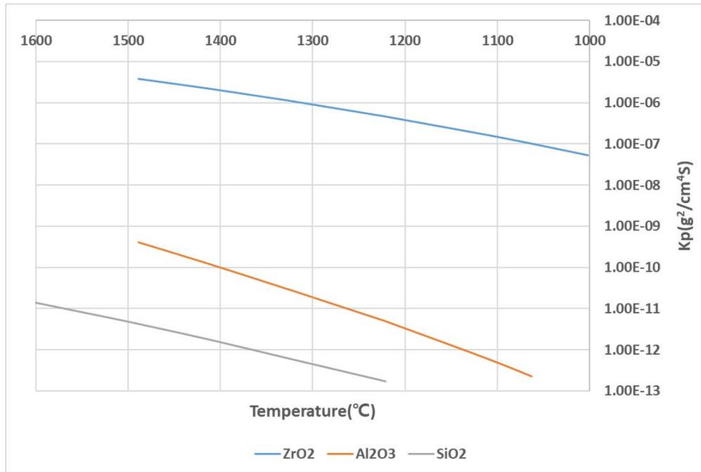
Fig 1. A rough comparison of parabolic rate constants of Zr, Al and Si (Ref 4.)
