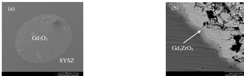
Fig. 5. Microstructure of 8YSZ pellets containing  $Gd_2O_3$  spheres; (a) SE image of the  $Gd_2O_3$  sphere and (b) BSE image of the interface between  $Gd_2O_3$  sphere and 8YSZ.
