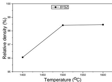
Fig. 1. Densification of 8YSZ by MW
