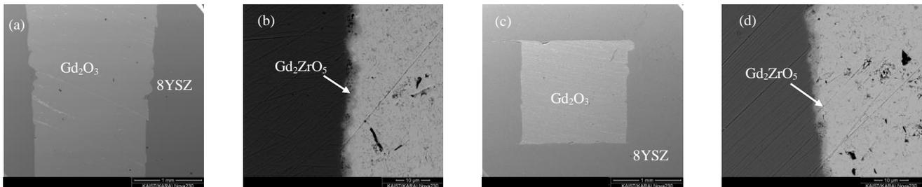
Fig. 3. Microstructure of 8YSZ pellets containing Gd<sub>2</sub>O<sub>3</sub> rod and minipellet; (a) SE image of Gd<sub>2</sub>O<sub>3</sub> rod, (b) BSE image of Gd<sub>2</sub>O<sub>3</sub> rod-8YSZ interface, (c) SE image of Gd<sub>2</sub>O<sub>3</sub> minipellet, and (d) BSE image of Gd<sub>2</sub>O<sub>3</sub> minipellet-8YSZ interface.
