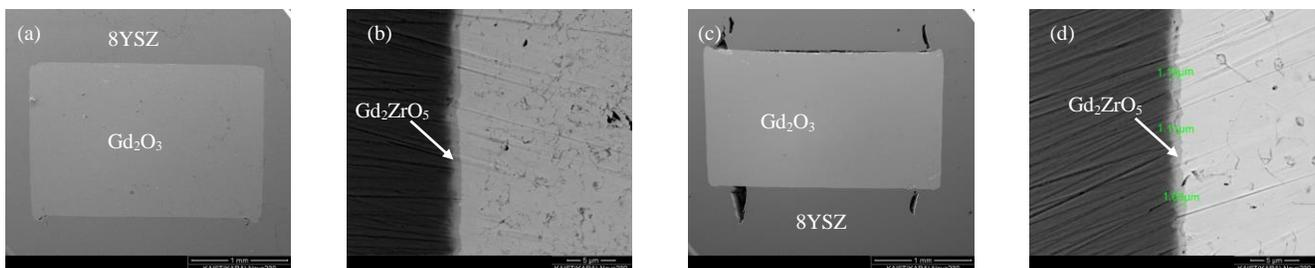
Fig. 4. Microstructure of 8YSZ pellet containing Gd<sub>2</sub>O<sub>3</sub> minipellet; (a) SE of CIPressed minipellet, (b) BSE image of CIPressed minipellet-8YSZ interface, (c) SE of sintered minipellet, and (d) BSE image of sintered minipellet-8YSZ interface.
