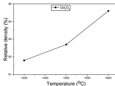
Fig. 2. Densification of Gd<sub>2</sub>O<sub>3</sub> by MW.
