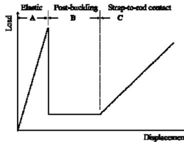
Fig. 6. Load-displacement schematic behavior in static analysis
