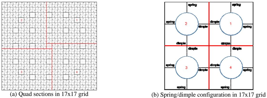
Fig. 4. Spring/dimple configuration for 17x17 array
