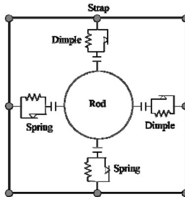
Fig. 1. Developed FE model concept of 1x1 grid
