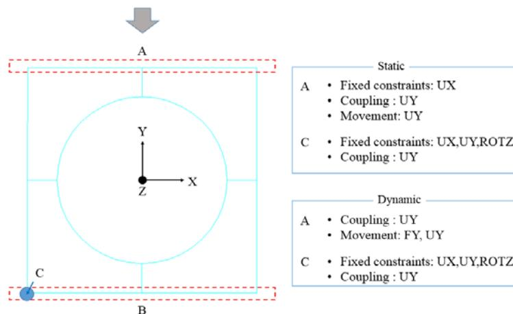
Fig. 3. Coupling and constraints condition
