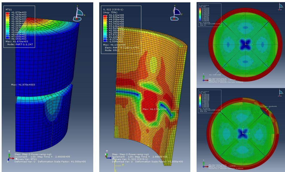
Fig. 1 Example of missing pellet chip model: left - calculated temperature distribution (3D model), middle - calculated hoop stress in cladding (3D model), right - calculated hoop stress no chip vs. chip (2D model).
