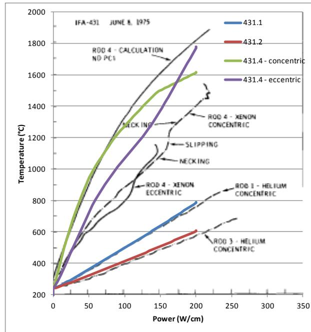
Fig. 6 Measured (black lines) and calculated (colored lines) temperature in the pellet centre as a function of power.
