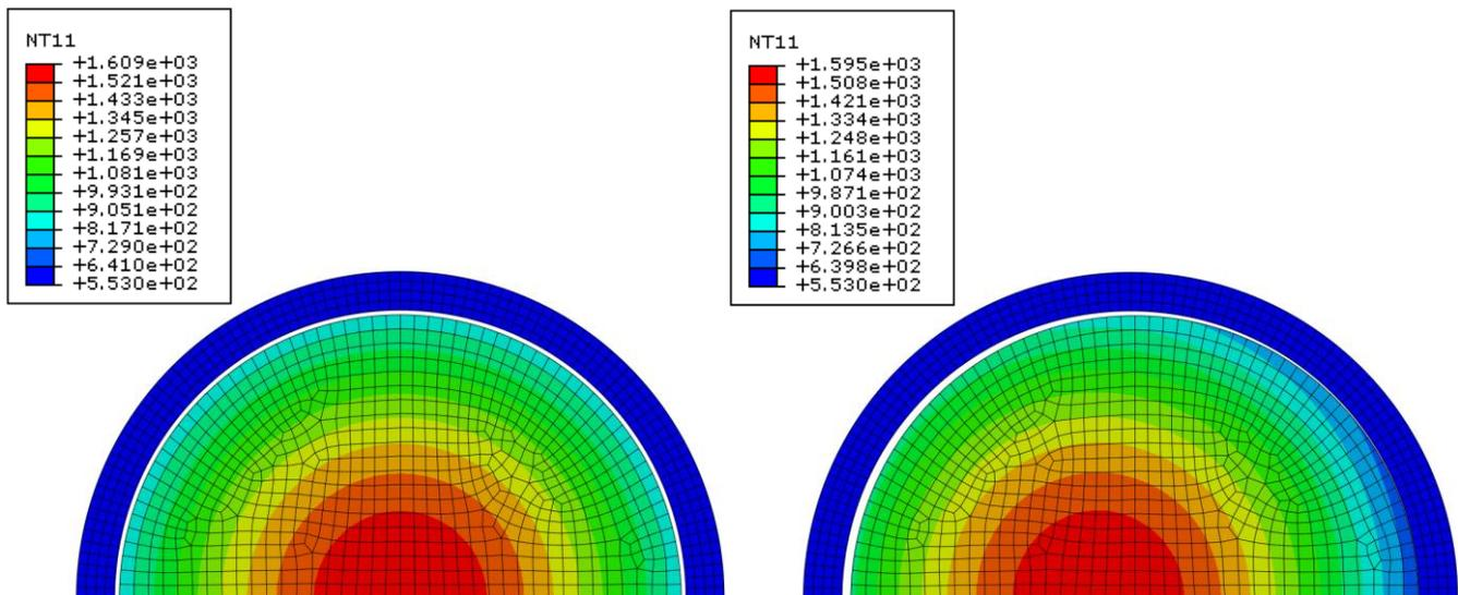
Fig. 2 Calculated temperature for central (left) and off-center (right) solid pellet stationary position in the cladding (temperature scale in Kelvins).
