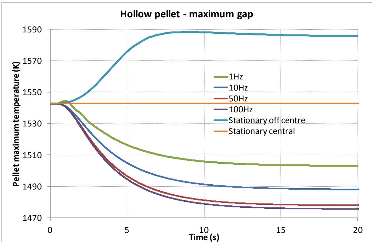
Fig. 4 Time evolution of maximum temperature (hollow pellet with maximum pellet-cladding gap) for different vibration frequencies.
