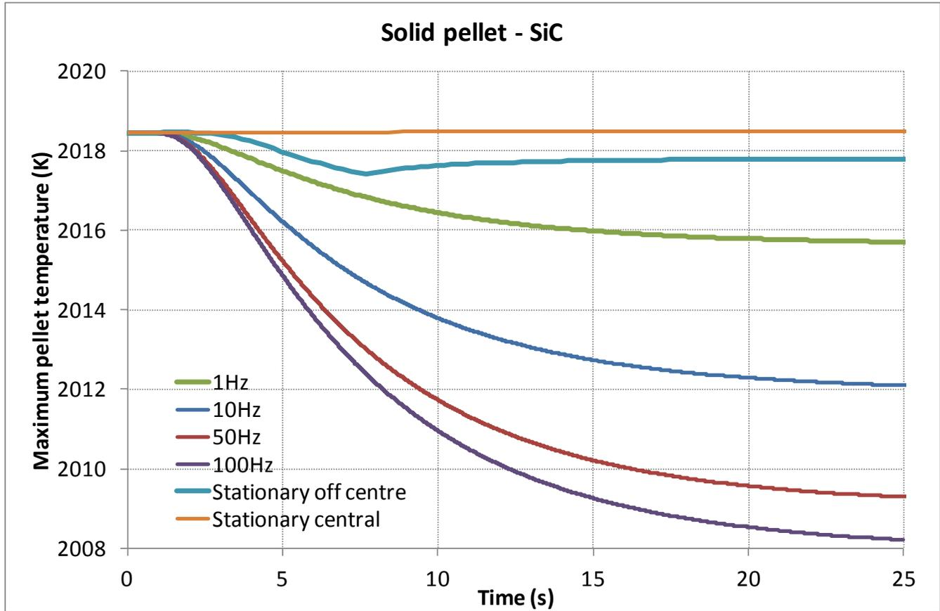
Fig. 5 Time evolution of maximum temperature (SiC cladding, solid pellet, 40 microns radial pellet-cladding gap) for different vibration frequencies.
