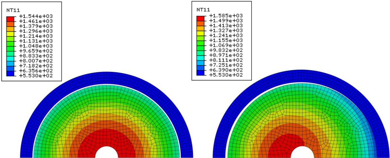
Fig. 3 Calculated temperature for central (left) and off-center (right) hollow pellet stationary position in the cladding (temperature scale in Kelvins).
