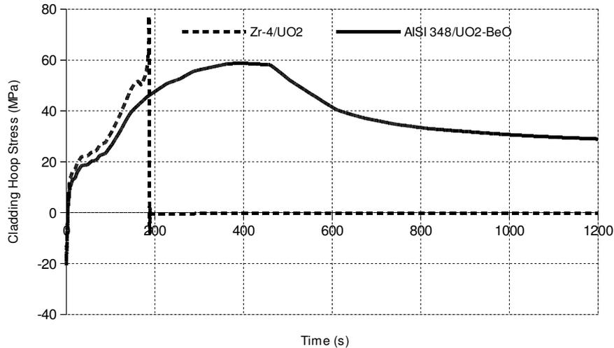
Fig. 8. Cladding hoop stress evolution under LOCA as function of time for IFA-650.5 test case considering Zr-4/UO<sub>2</sub> fuel system and AISI 348/UO<sub>2</sub>-BeO fuel system.
