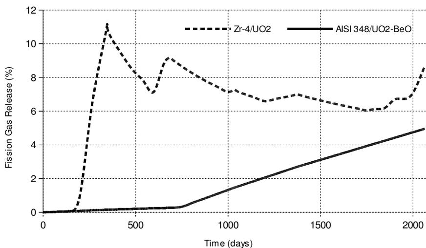
Fig. 4. Fission gas release evolution under steady-state irradiation as function of time for IFA-650.5 test case considering Zr-4/UO<sub>2</sub> fuel system and AISI 348/UO<sub>2</sub>-BeO fuel system.
