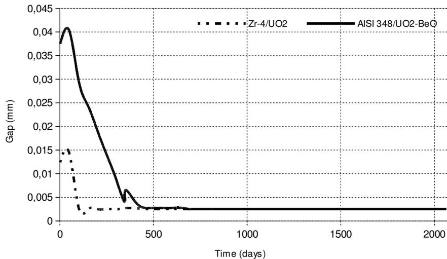
Fig. 5. Gap evolution under steady-state irradiation as function of time for IFA-650.5 test case considering Zr-4/ $\text{UO}_2$  fuel system and AISI 348/ $\text{UO}_2$ -BeO fuel system.
