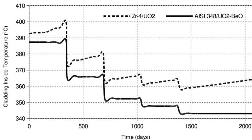
Fig. 2. Cladding inside temperature evolution under steady-state irradiation as function of time for IFA-650.5 test case considering Zr-4/ $\text{UO}_2$  fuel system and AISI 348/ $\text{UO}_2$ -BeO fuel system.
