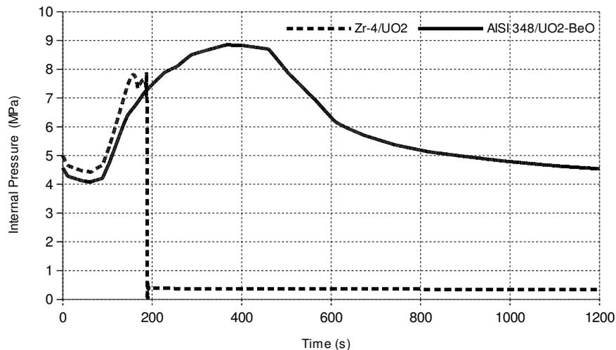
Fig. 7. Fuel rod internal pressure evolution under LOCA as function of time for IFA-650.5 test case considering Zr-4/ $\text{UO}_2$  fuel system and AISI 348/ $\text{UO}_2$ -BeO fuel system.
