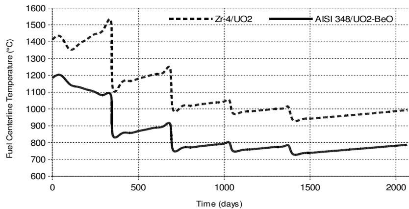
Fig. 1. Fuel centerline temperature evolution under steady-state irradiation as function of time for IFA-650.5 test case considering Zr-4/ $\text{UO}_2$  fuel system and AISI 348/ $\text{UO}_2$ -BeO fuel system.
