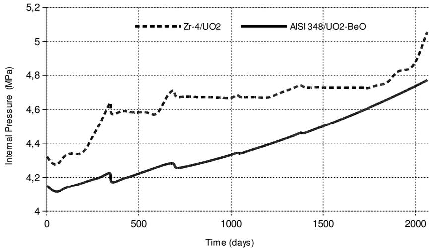
Fig. 3. Internal pressure evolution under steady-state irradiation as function of time for IFA-650.5 test case considering Zr-4/UO<sub>2</sub> fuel system and AISI 348/UO<sub>2</sub>-BeO fuel system.
