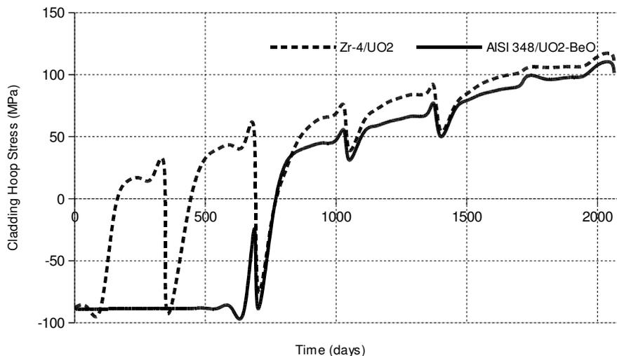
Fig. 6. Cladding hoop stress evolution under steady-state irradiation as function of time for IFA-650.5 test case considering Zr-4/ $\text{UO}_2$  fuel system and AISI 348/ $\text{UO}_2$ -BeO fuel system.
