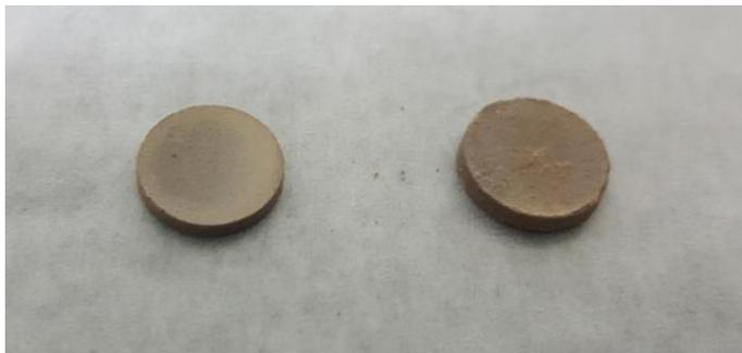
Fig. 2. Figure of CeO<sub>2</sub>-based hybrid pellets fabricated by microwave sintering at 1500 °C for 1 hour.
