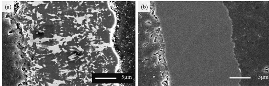
Fig. 1. Polished surface of (a) SiC and ZrC composite coating layer. (b) SiC matrix coating with ZrC particles.
