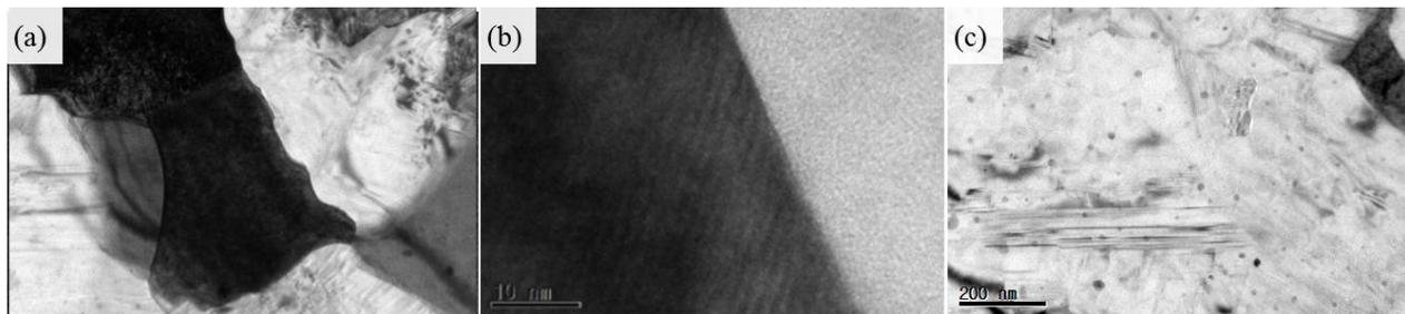
Fig. 2. TEM images of (a) SiC and ZrC composite coating layer, (b) SiC matrix coating with ZrC particles.
