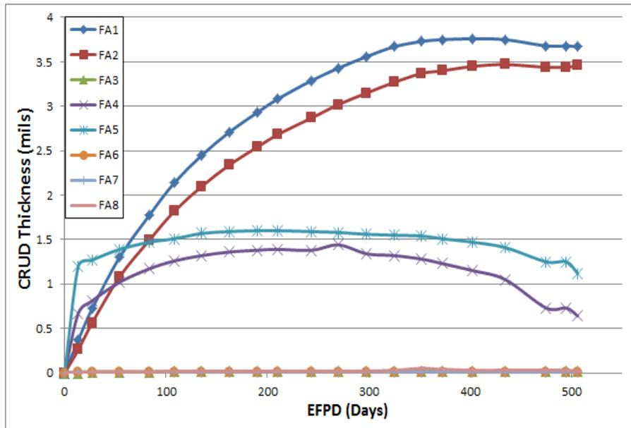
Fig. 2 Crud thicknes calculated by BOA code
