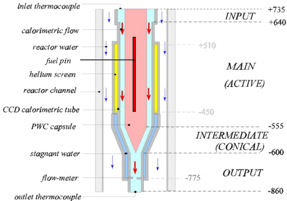
Fig. 1. Schematic overview of the Pressurized Water Capsule and Calorimetric Device to be used for the ATTICUS irradiation.
